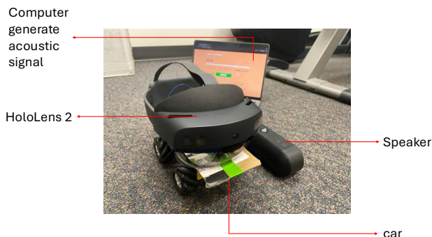
Figure 5: Experimental setup with XR headset, speaker and sound source, and remote-control car for mobility.
